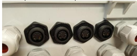
Figure 62 – Four Modbus IP67 sockets.
